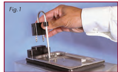
Detachable temperature probe.
