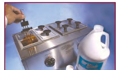
Tinting is simply done by dipping lenses into hot dye solution.
